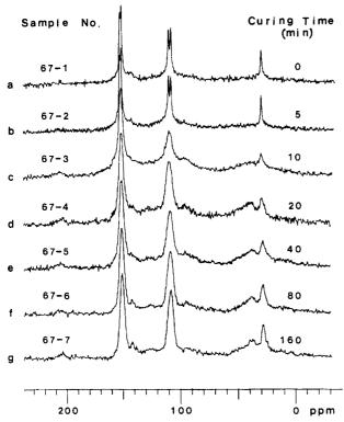
**Figure 1.** 15.0-MHz  $^{13}$ C CP/MAS spectra of the seven furfuryl alcohol resins, with 1-ms CP contact time and 1-s repetition time (number of scans: 8000–77000): (a) resin 67-1; (b) resin 67-2; (c) resin 67-3; (d) resin 67-4; (e) resin 67-5; (f) resin 67-6; (g) resin 67-7.
