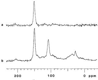
Figure 2. 15.0-MHz <sup>13</sup>C CP/MAS interrupted-decoupling spectra of resin 67-5, with 1-ms CP contact time and 1-s repetition time: (a) 100-µs interrupted decoupling, 40 560 scans; (b) usual CP/MAS spectrum, 21 560 scans.
